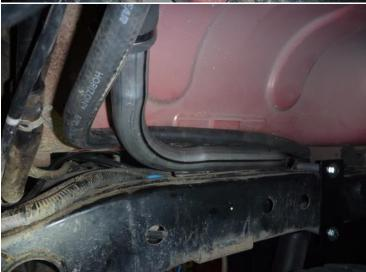
25. Double check all fuel line clamps and ensure the fuel lines are secure. Road test and check for rattlers & squeaks.
